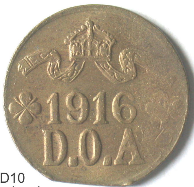
H6-D6 piece broken off H-die
